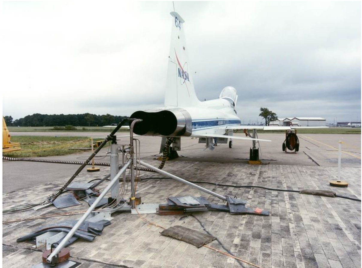
Inlet Probes Positioned 1 m behind LaRC T-38 with J-85GE engines
